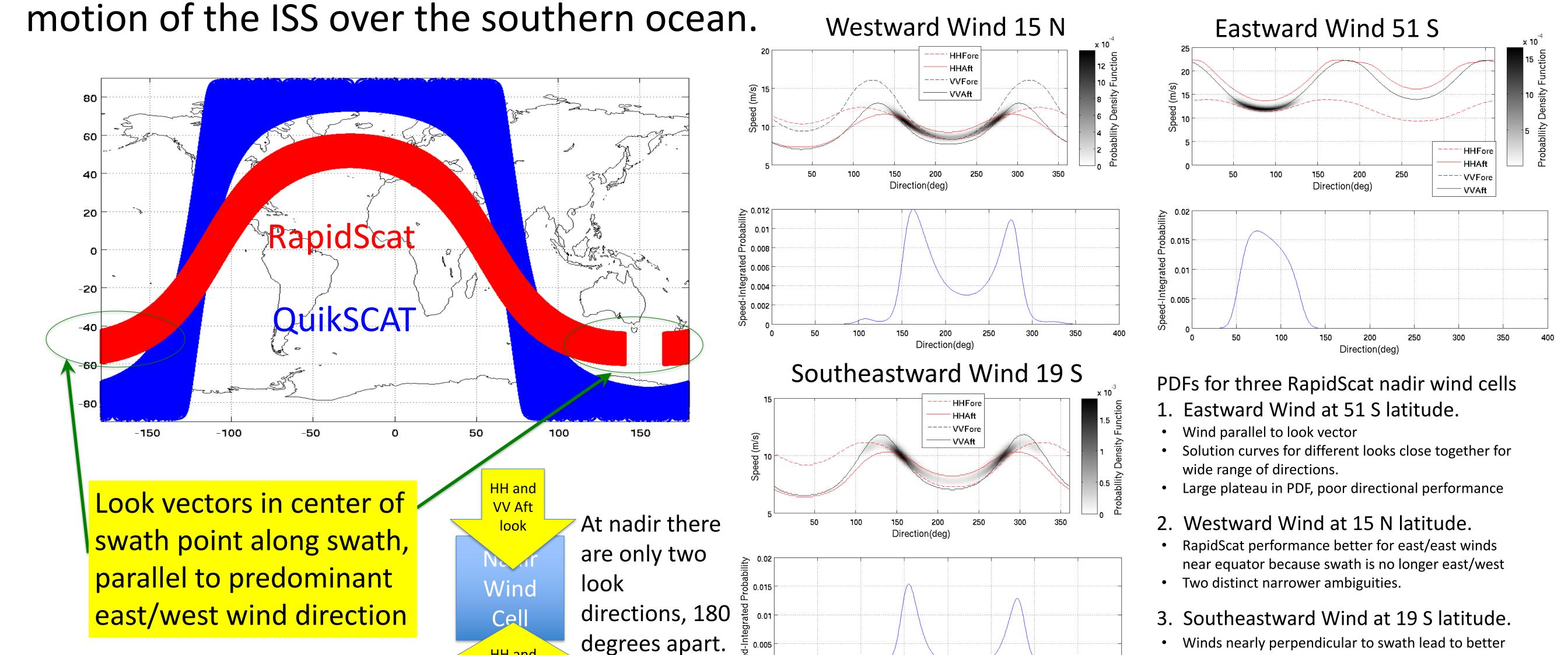
Errors in incidence angle dependency of GMF are also important sources of systematic directional error for RapidSCAT.
